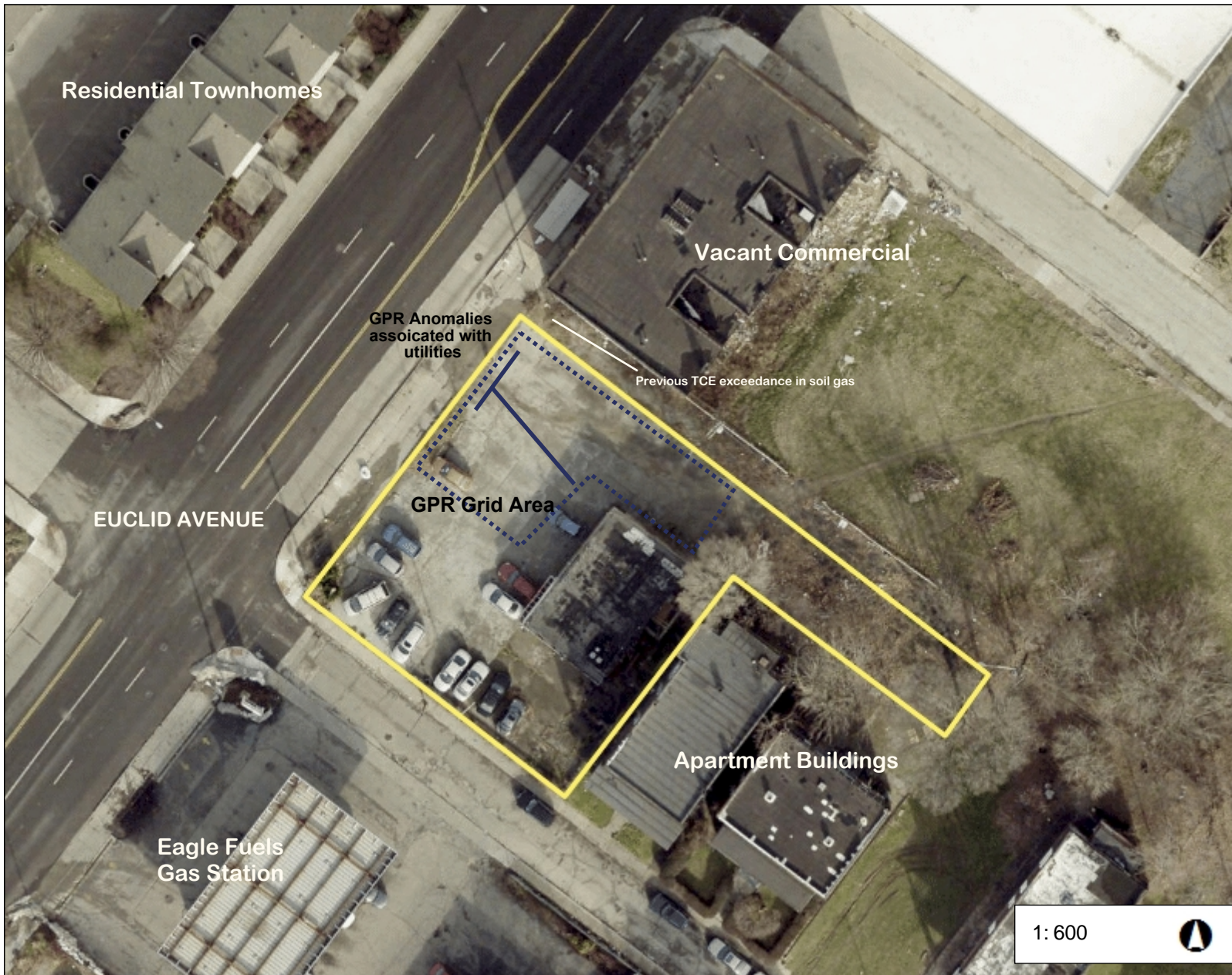
Figure 4: GPR Grid and Anomalies
