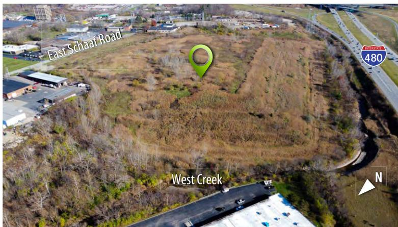
Creek that runs along the toe of the landfill. The cost to re-establish the top and side cap is estimated to be close to \$1.5M. Virtually all of the gas and groundwater monitoring wells have fallen into disrepair. Cost to repair will be about \$475K. Even after the 8 year period, the slope, cap and methane release will need to be monitored.
